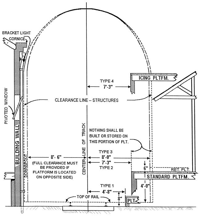
**EXEMPTION:** Except for handrail and water barrel clearances, the clearance requirements in Table 3 do not apply to bridge decks where railroad employees couple or uncouple cars on a switching lead unless the department approves them.
