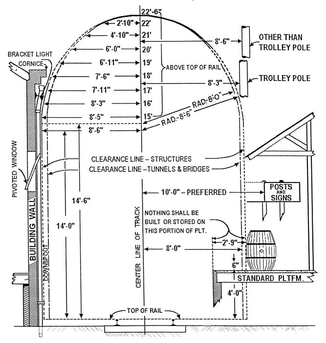
Illustration 3A - Minimum Side Clearance for Certain Structures in or on the Lower Sections of Bridges and Tunnels
